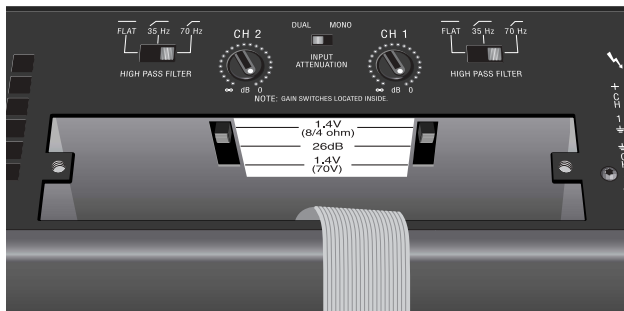
Figure 5.1 Input Sensitivity Switches for CTs 600/1200
